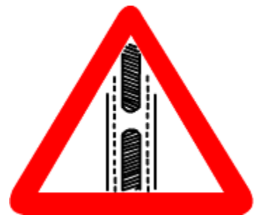
Gap in median
